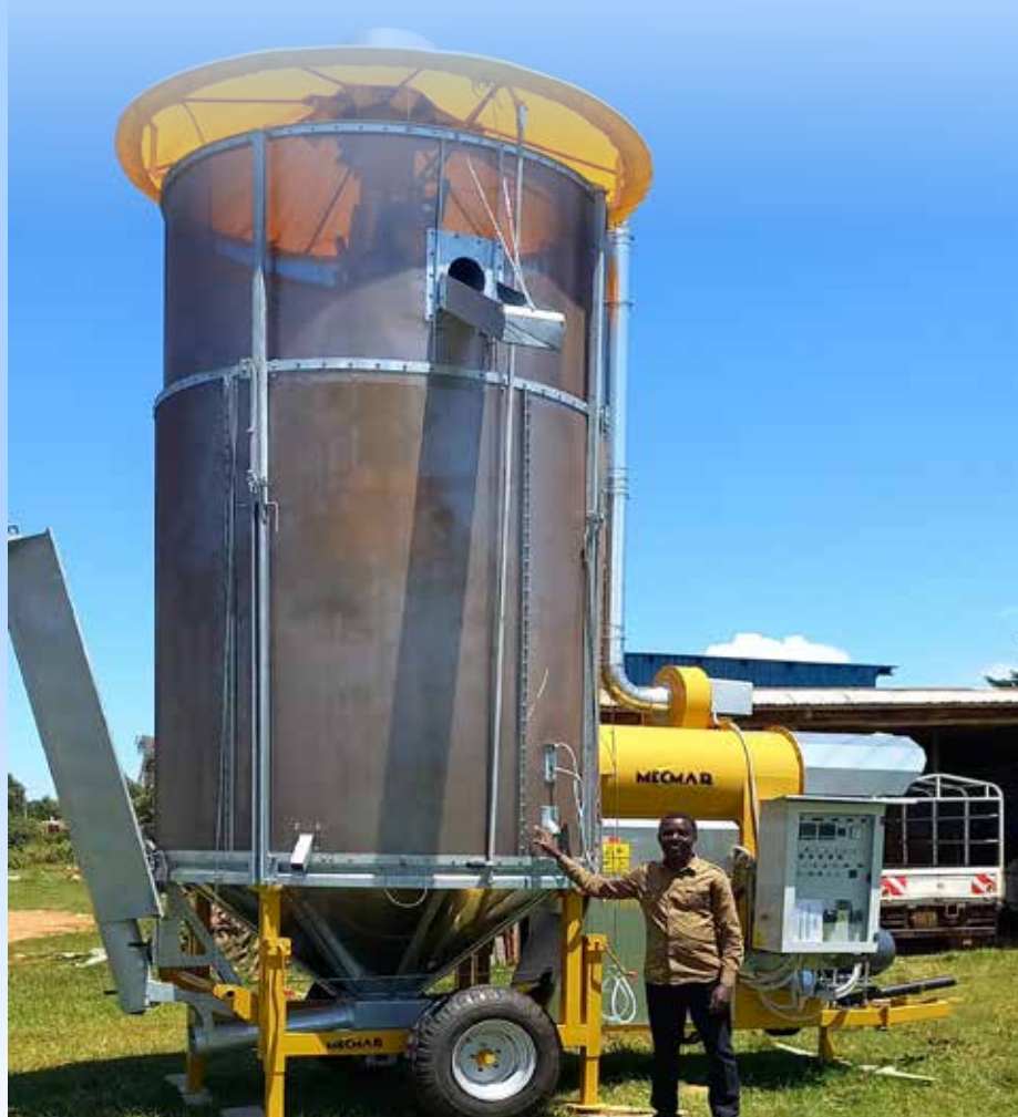
The silos are hermetic [airtight] and are made from metal sheets, making them rodent-proof and insect-proof, and use smart sensors to monitor critical storage conditions such as temperature, moisture, and air circulation. Photo Credit: Silo Africa
